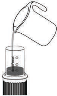
6 Add water up to ① on the chamber, 175°F (80°C) water for hot brewing or room temperature water for cold brew.
